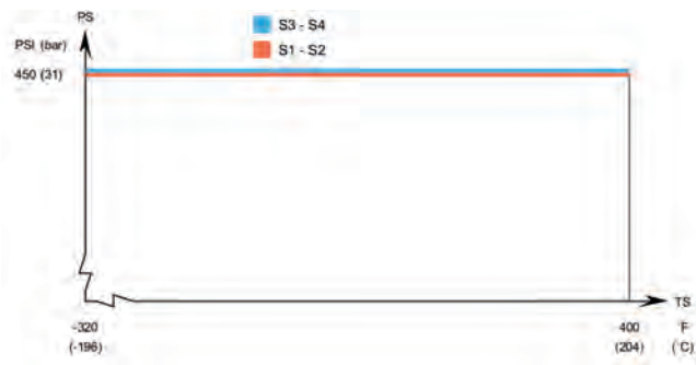
DOC60 - UL approval pressure/temperature graph*
