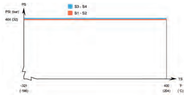
DOC112 - UL approval pressure/temperature graph
