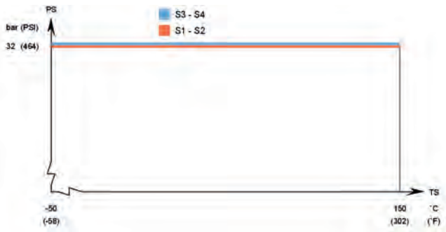
CB18 - UL approval pressure/temperature graph*
