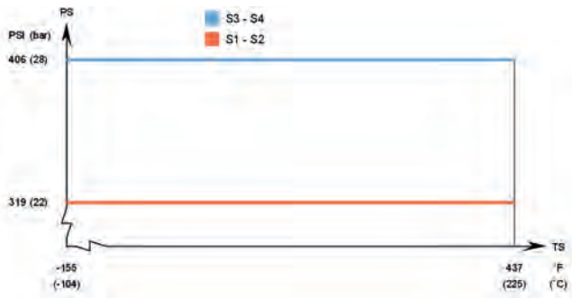
CB300 - UL approval pressure/temperature graph*
