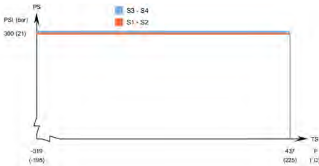
AlfaNova 14 - CRN approved pressure/temperature graph
