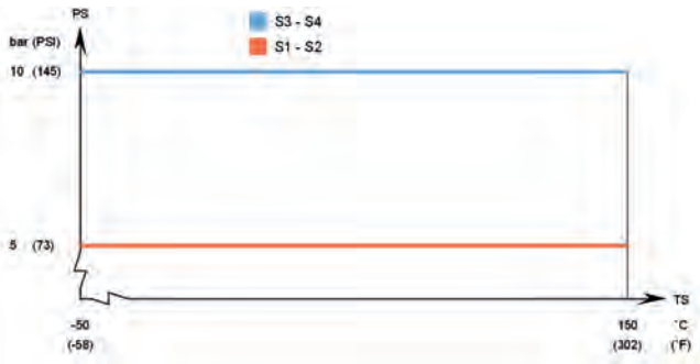
CBH18 - PED approval pressure/temperature graph* H
