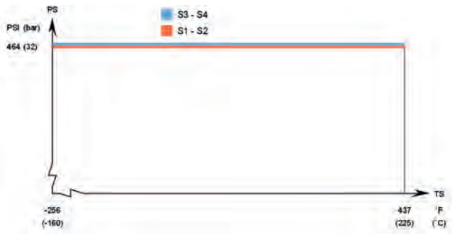
CBH16 - UL approval pressure/temperature graph*
