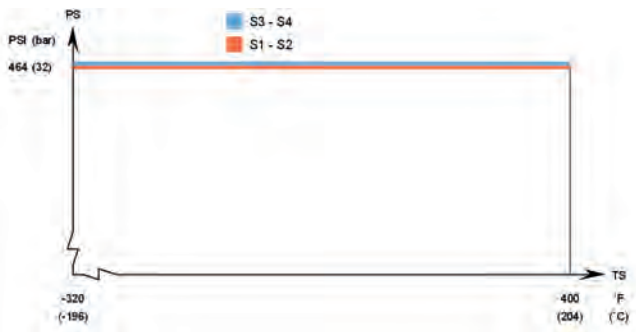
CB400 - CRN approval pressure/temperature graph*
